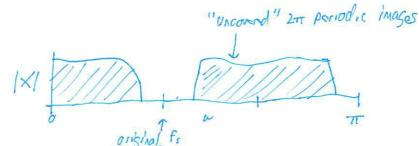
The following sinc interpolation filter will repair the spectrum of the upsampled signal:
