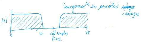
The following sinc interpolation filter will repair the spectrum of the upsampled signal:
