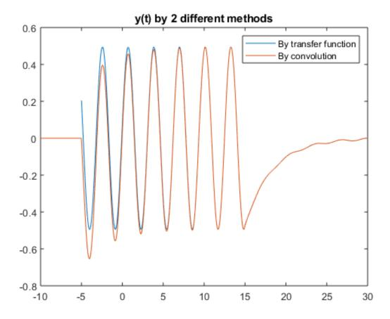
These approaches agree in the central portion. Note that convolution diverges from the correct result at the edge. The main reason for this is that the input x(t) is implicitly taken as 0 outside the range where it is defined (t values). Additionally, there is some error since the right tail of h(t) is truncated.
