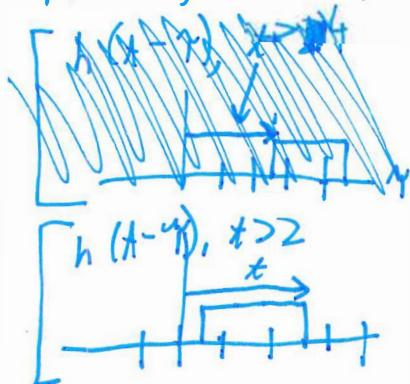
$$\begin{aligned} y(t) &= \text{area of } (x(\gamma) \cdot h(t-\gamma)) \\ &= \text{width} \times \text{height} \\ &= \int_{t-2}^2 1 \cdot 1 \, d\gamma = 2 - (t-2) = 4 - t \end{aligned}$$
