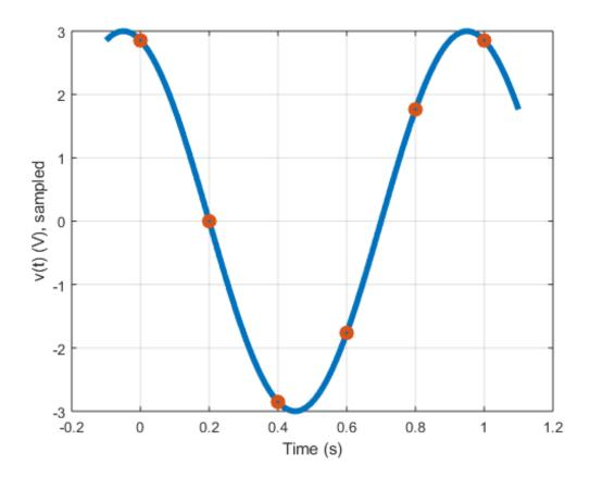
b. Then quantizing the signal (going from continuous/analog voltage) with a resolution of 0.5 V.
