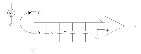
$$Q = C_{top}V_H - (C_{top} + C_{bot})V_i$$
