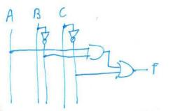
3. A point Re-draw it using just NAND and NOT gates in the most simplified SOP form.
